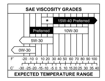
The use of correct oil viscosities for diesel engines is important for satisfactory operation. Determine which oil viscosity best suits the temperature range you expect to encounter for the next service interval.
